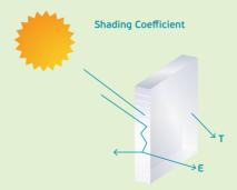
Shading co-efficient(SC): The ratio of total solar radiation through a particular glass type, relative to the total solar radiation through 3mm clear float glass. This show the glass performance in reducing heat.
